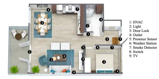
Figure 4.1. Floor plan of the experimental testbed
